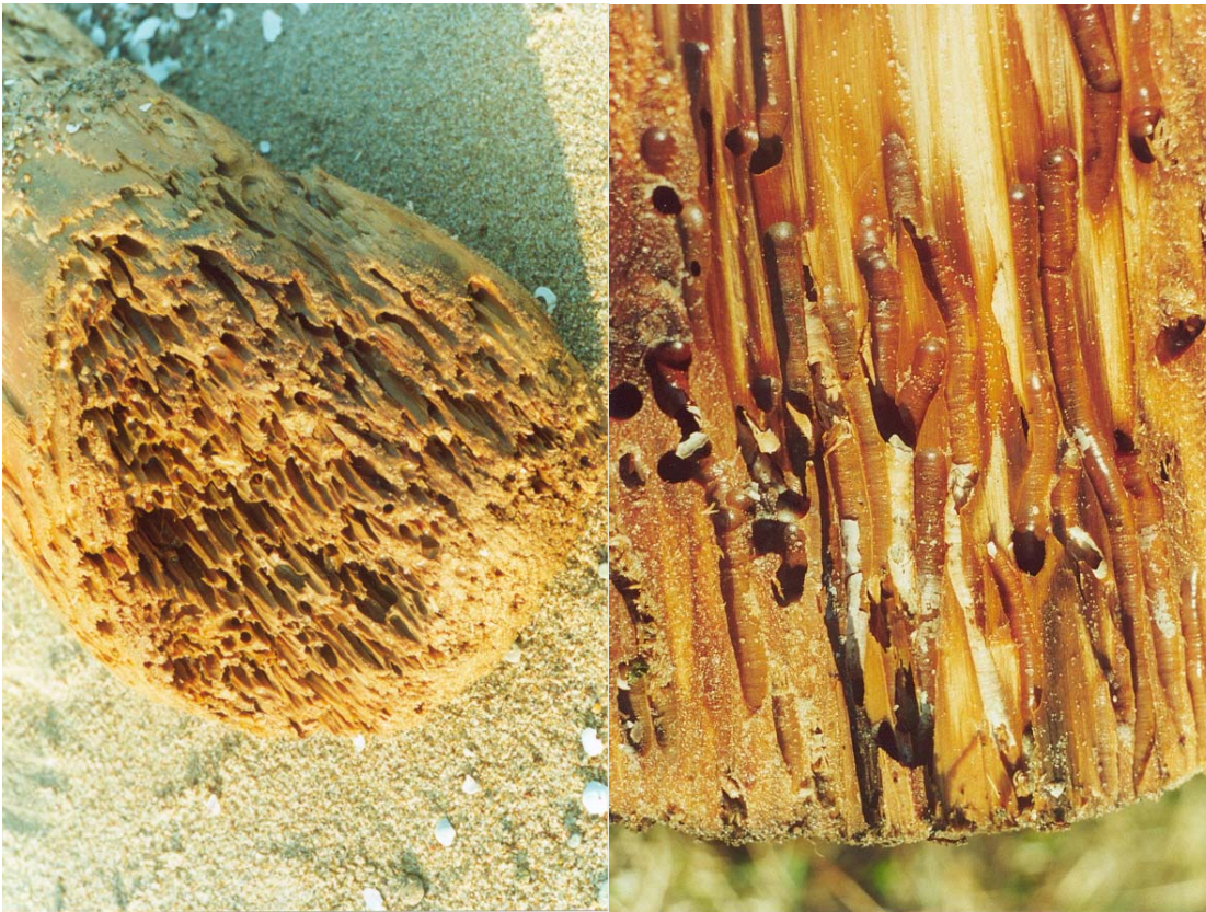
Fig 1 and 2. Pieces of wood (groyne piles) heavily damaged by shipworm can reach as far as the Lithuanian sandy beaches, travelling 500 km northwards from the northernmost fringe of the species' area of distribution. No specimen survived. Photos by V. Didžiulis. Chunks of wood found by Dr. J.
